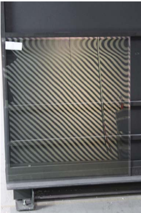
1. Viwinco Current 3mm Low-E Tempered Glass
