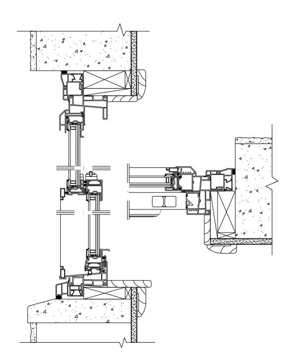
MASONRY OPENING - 1/2" = TTT CASING TTT CASING - 3.72 = FRAME WIDTH TTT CASING - 2.775 = FRAME HEIGHT
