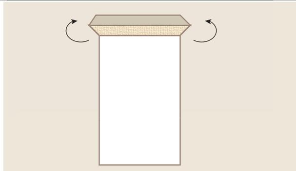
**6** Install flexible flashing tape across the bottom of the opening flexing it to go up each side approximately 6". Part of the flashing tape should extend into the opening. Form a sill dam with the back part of the tape that extends across the sill. If standard flash tape is used, apply the top edge of the flashtape even with the rough opening at the bottom, and extend the ends approximately 6" past the opening on either side.
