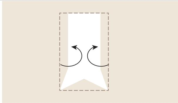
**4** Cut a diagonal line at top corners of window opening to create a flap approximately 6" above the top of window opening.
